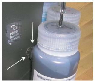
Velcro attaches bottles to printer (This is photo from a 2200 printer)
